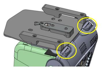
Place the mounting plate on the bottom of the defibrillator as shown above, make sure the front loops are hooked around the front feet of the defibrillator.
