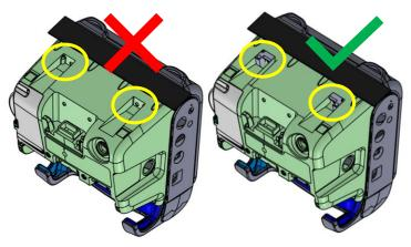
Check bottom of defibrillator for mounting hooks. If the mounting hooks are not present on the unit get them added then proceed.
