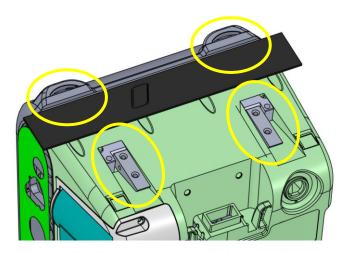
If the defibrillator has the side packs installed make sure the bottom strap is not overlapping the front foot.
