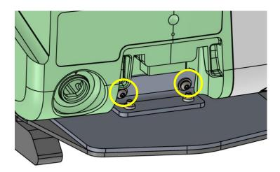
Tighten rear bracket screws to defibrillator to 15 lfb-in.
