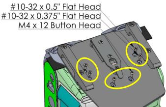
Apply Loctite 243 to the threads of all 6 screws used in this step.
