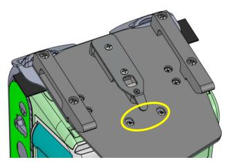
Tighten rear bracket screws to mounting plate to 15 lfb-in.
