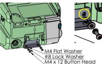
Attach the rear bracket using the indicated hardware. Note the fasteners are in the slotted holes in the rear bracket not the threaded hole. Fasteners should be screwed in until rear bracket touches defibrillator, do not tighten.
