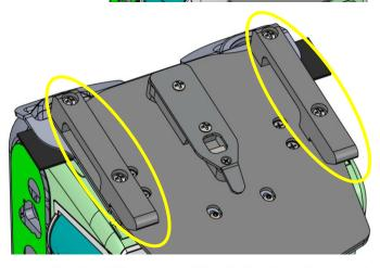
Grab the stands on the bottom of the mounting plate and pull to check the mounting plate is securely attached to the defibrillator.
