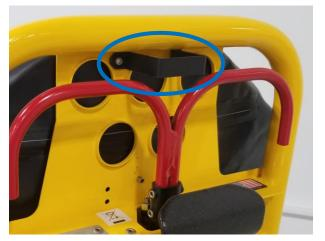
Install backrest release cover using the dome head rivets.
