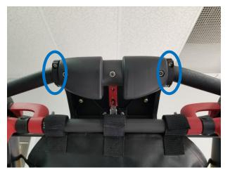
Install front clamps using 10-32 x 3/8 socket head cap screws. Use Loctite on fasteners.
