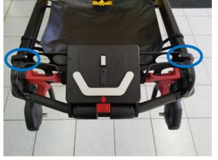
Place dock on cot as shown. Install side U clamps using 10-32 x 3/8 socket head cap screws. See picture to right for spacer orientation. Do not tighten fasteners yet. Use Loctite on fasteners.
