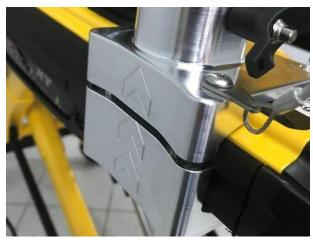
Push the block up and add the securing bolts
