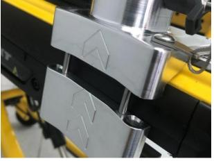
Add the lower block assembly lining up the guide pins – then adding the bolts provided
