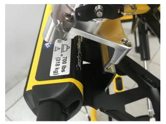
With lower portion of block removed and screws loosened off. Hook the stainless steel bracket over the black support bracket
