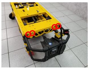
Remove fasteners indicated by the red circles in existing deck.
