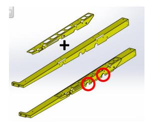
Place the R-800494 Right Inner Side Rail inside the R-800495 Right Outer Side Rail. Make sure the cut outs indicated by the red circles are aligned.
