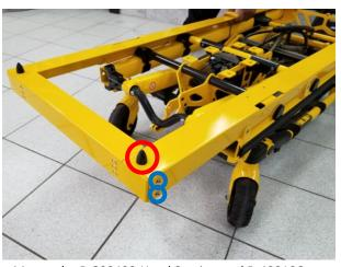
Mount the R-800499 Head Section and R-400106 Bumper to the Outer Side Rails using R-102165 #10 flat washer and R-102160 10-32 x % Button Head where indicated with the blue circles. In the red circle use a R-102164 % Flat Washer and R-102158 % x % Button Head for the Bumper. Do the same for the other side. Do not tighten any fasteners.
