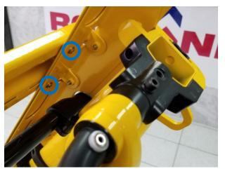
Finish attaching the R-800498 Cross Bars with a R-102165 #10 Flat Washer and R-102161 10-32 x ¾ Button Head in the 2 locations indicated with the blue circle. Do this on both sides of both Cross Bars.
