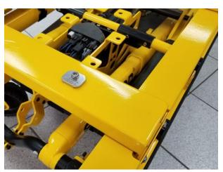
Place isolette on top of the Cross Bars and insert the R-800500 Threaded Plate into the mounting locations on the isolette. Secure the isolette with a R-102166 5/16 Flat Washer and R-102162 5/16 x 1.25 Button Head.
