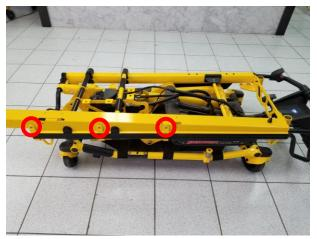
Mount the Right Outer and Inner Side Rails to cot with R-102158  $\frac{1}{4}$  x  $\frac{1}{2}$  Button Head Screws where indicated with red circles. Do not tighten fasteners.
