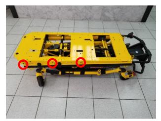
Remove fasteners indicated by the red circles in existing deck.
