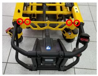
Mount the Right Outer and Inner Side Rails to cot with R-102164  $\frac{1}{4}$  flat washers and R-102159  $\frac{1}{4}$  x  $\frac{1}{4}$  Button Head Screws where indicated with red circles. Do not tighten fasteners.
