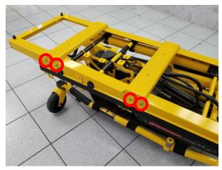
Mount the two R-800498 Cross Bars using a R-102164 ¼ Flat Washer and R-102159 ¼ x ¾ Button Head where indicated with a red circle. Do not tighten any fasteners.
